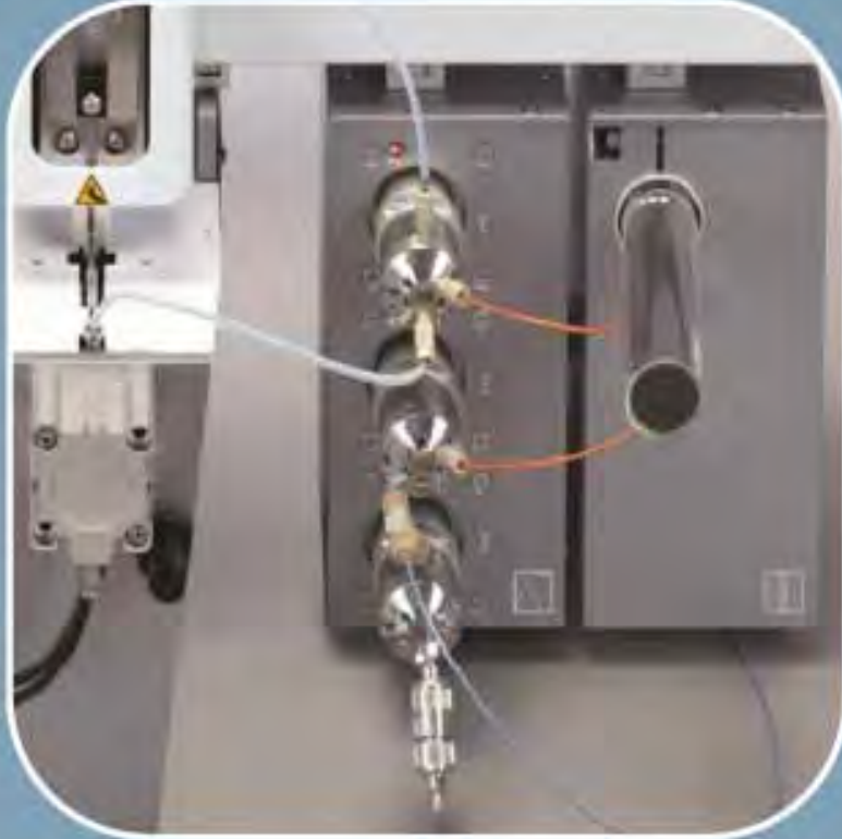
SCAP clamp module connected to Valve Module and Ultrasonic Module
