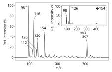
Figure 4 - Full SICRIT<sup>®</sup> mass spectrum and  $MS^2$  transition (154 to 126; see inset) of DEPA measured on the Mini 10.5 MS.
