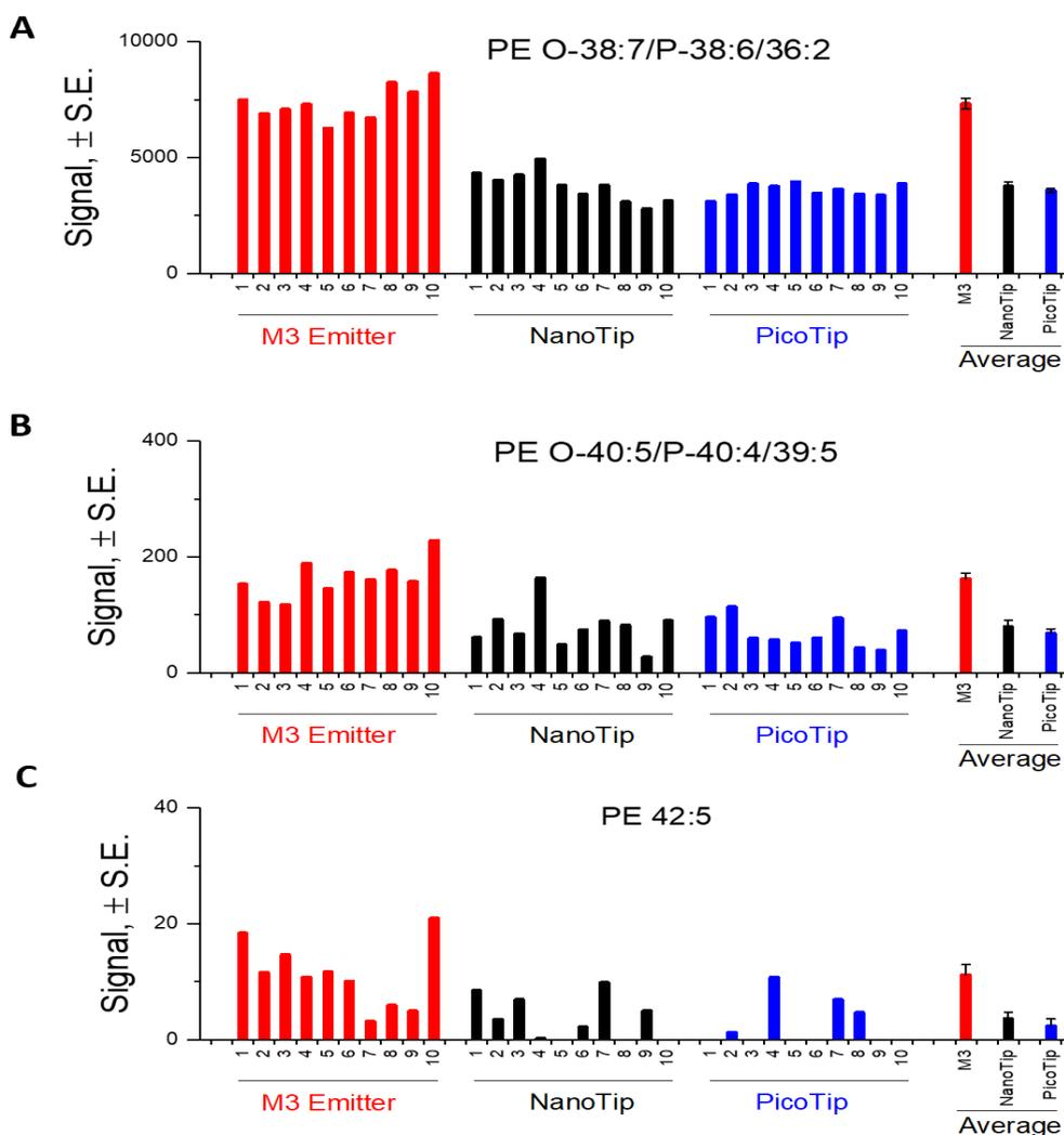
**Figure 2.** Representative TIC signals of PE species obtained using different type of emitters. The exactly same plasma lipid samples were infused into the mass spectrometer and the signals were acquired. We performed 10 consecutive injections using M3 emitter, NanoTip, and PicoTip, respectively. **A.** The most abundant PE species detected in plasma. **B.** The medium abundant PE species in plasma. **C.** The least abundant species in plasma.
