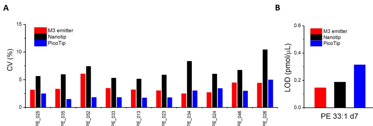
**Figure 4.** Reproducibility and detection limit of PE species by ESI-MS using M3, NanoTip, and PicoTip emitters. **A.** CV of the signals of the 10 most abundant PE species (n=10). **B.** LOD for one representative PE species PE 33:1 d7 for three types of emitters.
