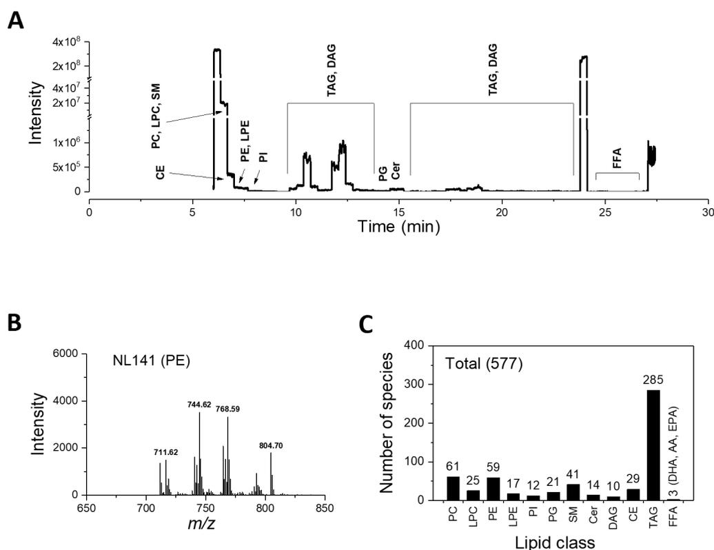
**Figure 1.** Shotgun lipidomics of pooled human plasma showing identification and quantification of 577 lipid species. **A.** TIC of lipid spectra acquired by direct infusion ESI-MS of one sample. Each lipid class was scanned in a separate segment. **B.** Spectra of the neutral loss 141 scan for PE species. **C.** Number of lipid species in each of the 12 lipid classes that were identified and quantified using our shotgun lipidomics platform.
