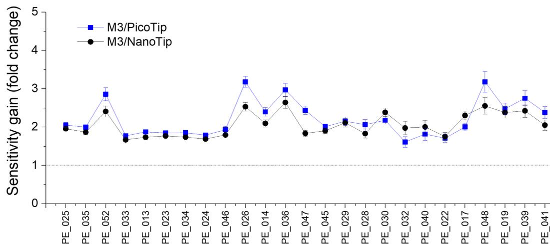
**Figure 3.** Sensitivity gain of ESI-MS using M3 emitter compared to single-nozzle emitters on the most abundant 25 PE species in human plasma. The signals of PicoTip and NanoTip emitters were used as denominators. On average, 2-fold increase in sensitivity was observed for M3 emitters.
