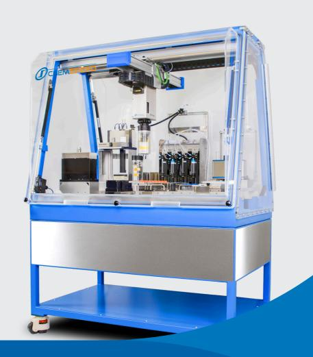
High-throughput library synthesis and reaction screening with online benchtop NMR (e.g. automated synthesis, online characterization, data analysis, AI / ML closed loop). The leading technology in overhead gravimetric dispensing / dosing (patented) combined with our various reactor formats for conventional, MW-assisted, reactive gas, photochem synthesis and our user-friendly software enable you to accelerate, standardize, digitalize your library synthesis and reaction screening workflows.
