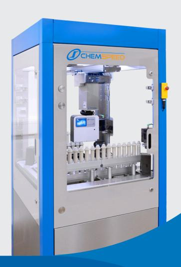
Automated, parallel library synthesis and reaction screening with online benchtop NMR (e.g. automated synthesis, online characterization, data analysis, AI / ML closed loop).
