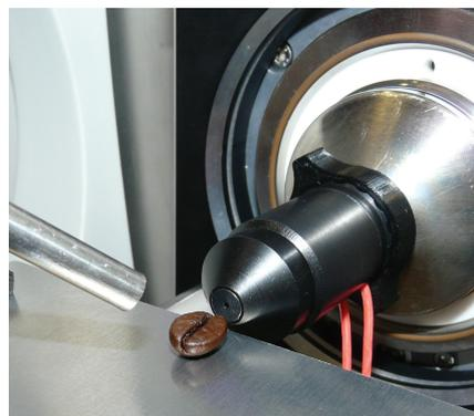
Figure 2 -Coffee aroma profiling by direct VOC desorption in front of the SICRIT® ion source
