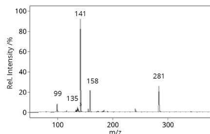
Figure 3 - Full SICRIT<sup>®</sup> mass spectrum of sarin with M+H (m/z 141), M-C<sub>3</sub>H<sub>6</sub> (m/z 99), M+H<sub>2</sub>O (m/z 158) and 2M+H (m/z 281) species acquired on the AB Sciex MS.
