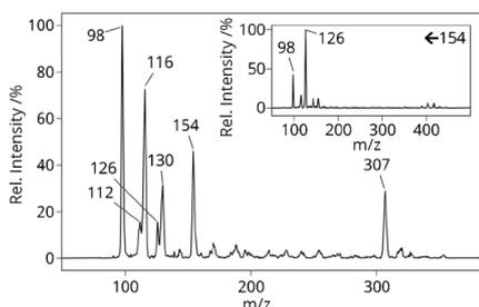
Figure 4 - Full SICRIT<sup>®</sup> mass spectrum and MS<sup>2</sup> transition (154 to 126; see inset) of DEPA measured on the Mini 10.5 MS.
