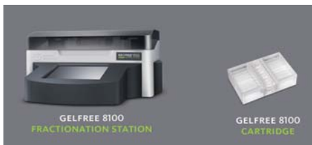
Figure 1. The Gelfree B100 instrument (left) is an eight channel electrophoretic controller that supplies voltage independently to each of the eight channels in the pre-cast cartridge (right). To use the system, the user programs the sequence (or chooses from a pre-programmed sequence) for each of the eight electrophoretic channels and starts the experiment. The device automatically pauses the experiment when each time interval has expired, allowing the user to extract the molecular weight fraction of interest. Measurement information for the eight channels is displayed to the user in tabular and graphical format during the course of an experiment.
