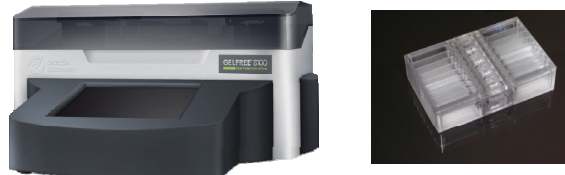
Figure 4: The GELFREE instrument (left) is an eight channel electrophoretic controller capable of simultaneously supplying constant current or voltage to each of the eight channels in the cartridge (right). A touch screen display located on the front of the instrument allows the user to program the voltage/current to apply to each cell, as well as the fraction entrapment intervals. To use the system, the user programs the sequence (or chooses from a pre-programmed sequence) for each of the eight electrophoretic cells and starts the experiment via the touch screen interface. The device automatically pauses the experiment whenever the time interval has expired, allowing the user to extract the molecular weight fraction of interest. Measurement information for the eight channels is displayed to the user in tabular and graphical format during the course of an experiment. Additionally, this run information is exportable in text delimited format using a USB port located on the back of the instrument.
