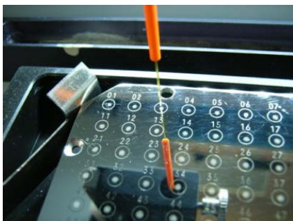
Figure 4 Biocompatible deposition needle
